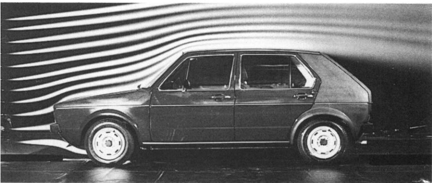
Figure 1.1 Streamlines in the longitudinal midsection of a VW Golf I (Rabbit), photographed for a full-sized vehicle in the large climatic wind tunnel of the Volkswagen AG. The lines of smoke were introduced in the plane of the longitudinal centreline to show the flow pattern with symmetrical oncoming flow. This flow state exists only when there is no side wind
