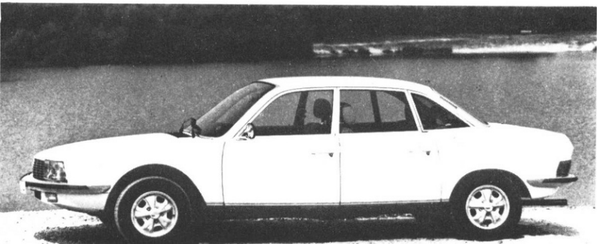
Figure 1.54 Top: Citroën GS, 1970, c_D = 0.38 (courtesy Citroën). Bottom: NSU Ro 80, 1976, c_D = 0.38 . Model launched 1967, c_D = 0.36 (courtesy Volkswagen AG)
