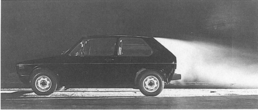
Figure 1.2 Wake of a VW Golf I, photographed as in Fig. 1.1, smoke introduced into the wake
