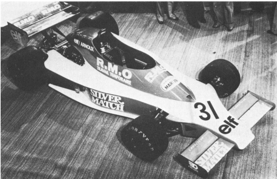
Figure 1.4 Negative lift wings on a Formula 1 racing car
